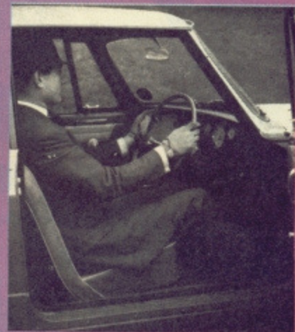
Fig. 19 The correct position: clear view of road ahead and legs not cramped or stretched
